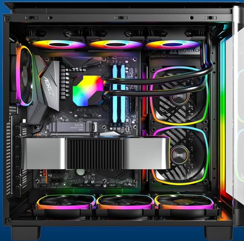
Figure 4.2: Example installation of the AIO cooler within a PC chassis.
