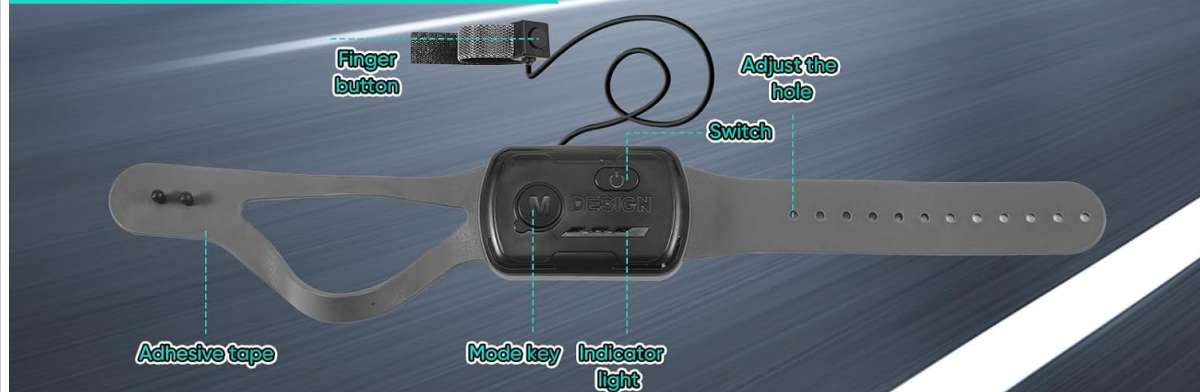
Figure 4: Remote Control and Gesture Sensing Watch layout.
