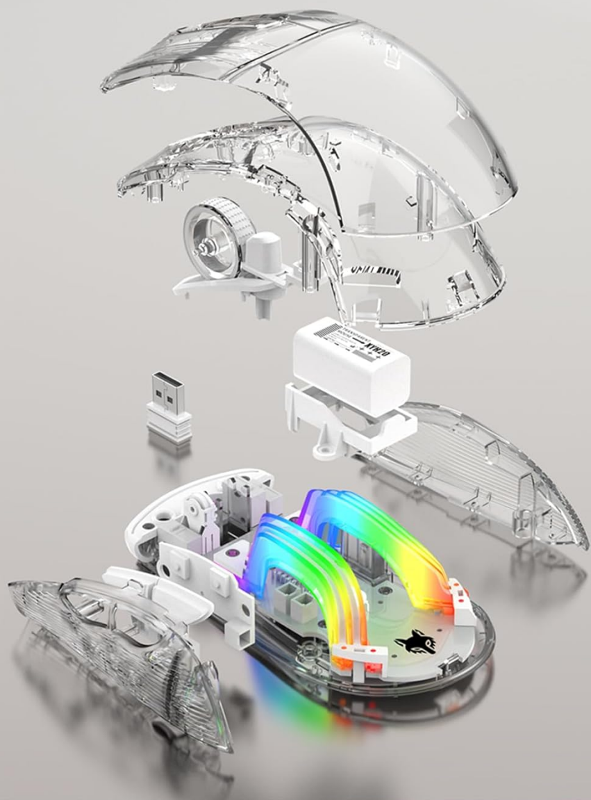
An exploded diagram of the XYH20 mouse, revealing its internal structure, circuit board, battery, and other components, demonstrating its layered construction.
