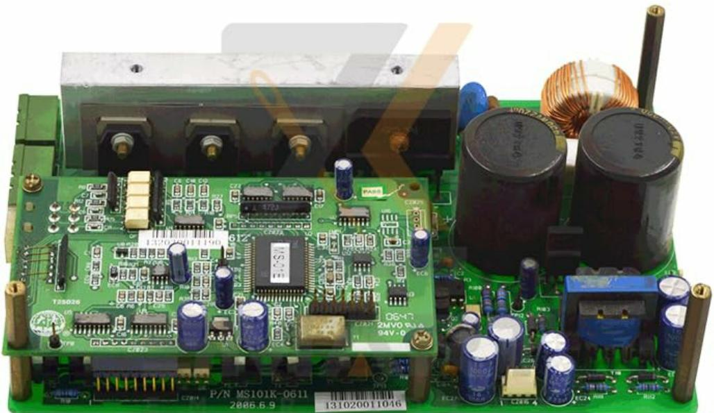
**Figure 1:** Phicus MS-02 Motor Driver Board. This image displays the compact electronic board with various connectors and components, typical of a motor driver for industrial embroidery machines.
