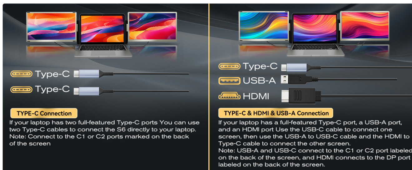
Image: Detailed connection diagrams for Type-C only and mixed Type-C/USB-A/HDMI setups.
