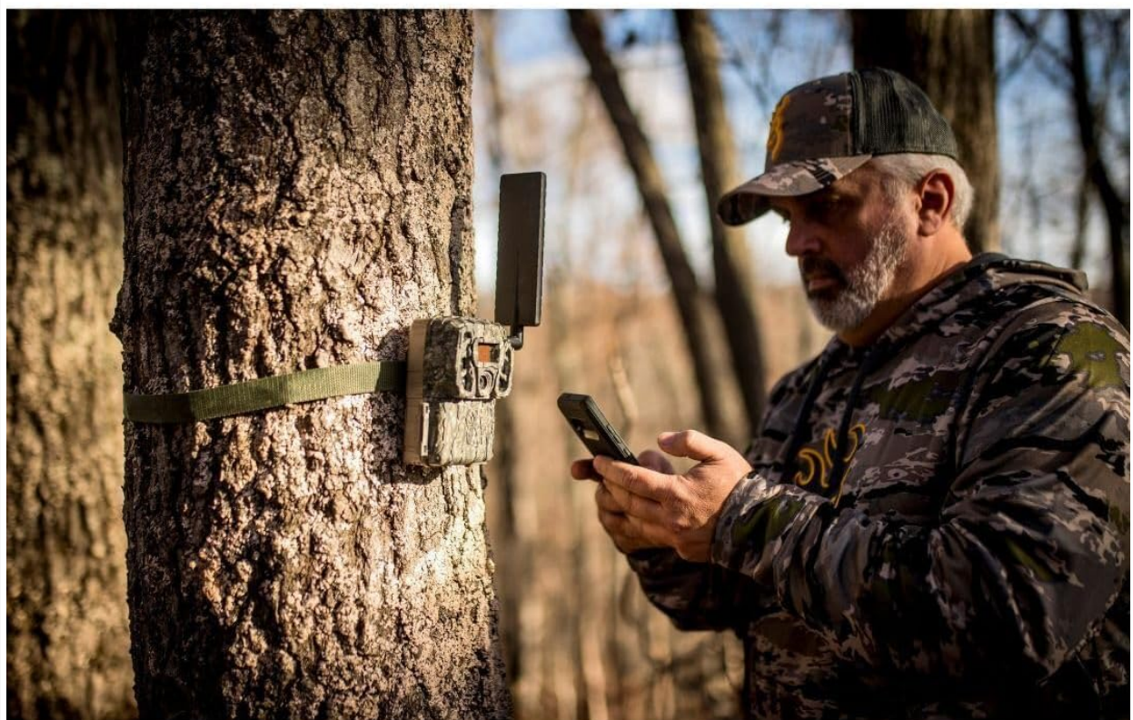
Figure 4.1: Camera Mounting. A person is shown adjusting the Browning Defender Vision Pro HD trail camera, which is mounted on a tree, while simultaneously interacting with a smartphone to manage settings remotely.
