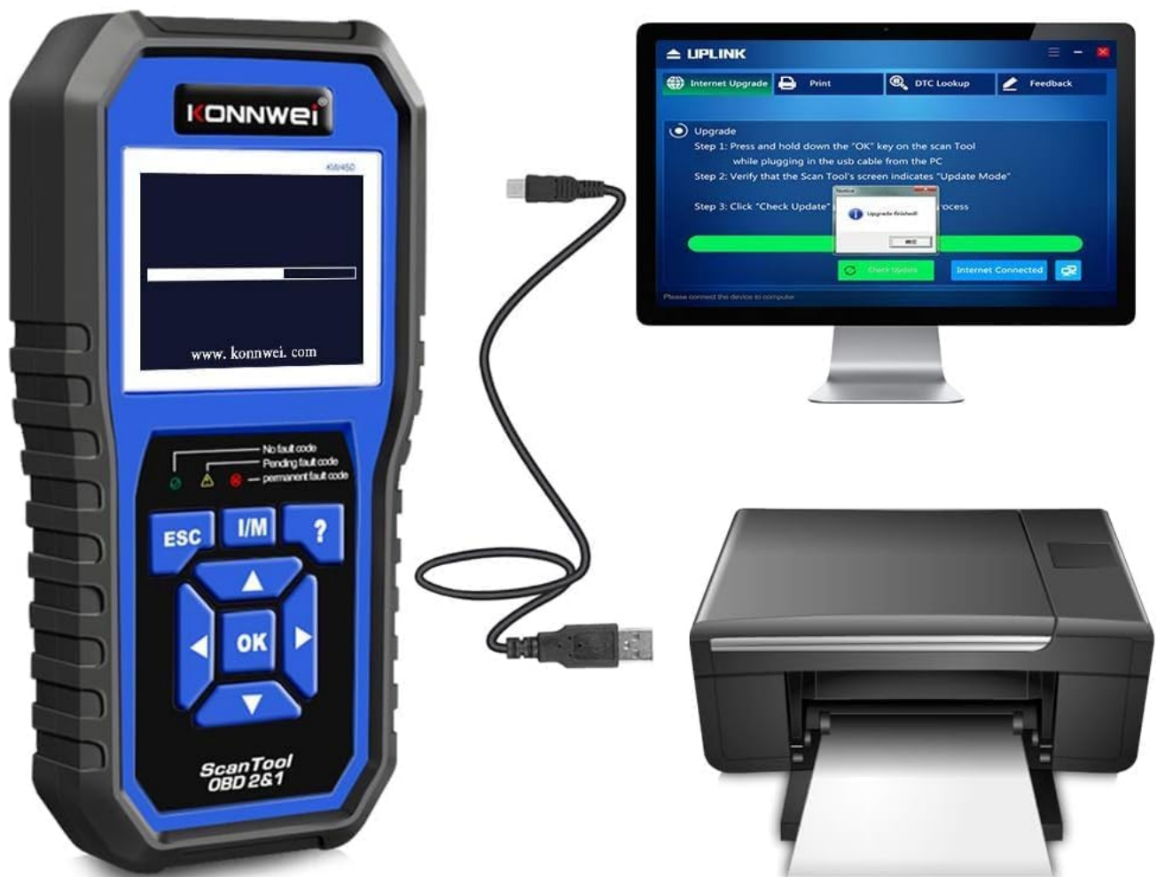
Figure 4: The KONNWEI KW450 main screen, showing indicators for 'No fault code', 'Pending fault code', and 'Permanent fault code' which are crucial for troubleshooting.
