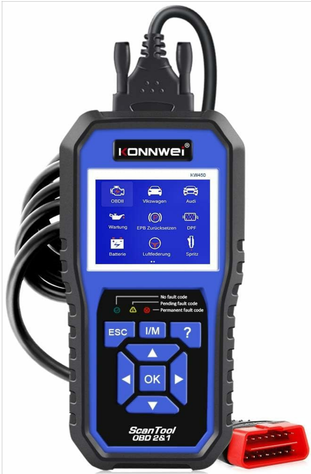
Figure 1: KONNWEI KW450 displaying its 9 special functions for VAG vehicles. These include Oil Service Reset, TPS Replacement Reset, Electronic Parking Brake (EPB) Reset, Battery Matching, Diesel Particulate Filter (DPF) Regeneration, Steering Angle Sensor (SAS) Calibration, Injector Coding, Suspension Adjustment, and Lamp Setting.
