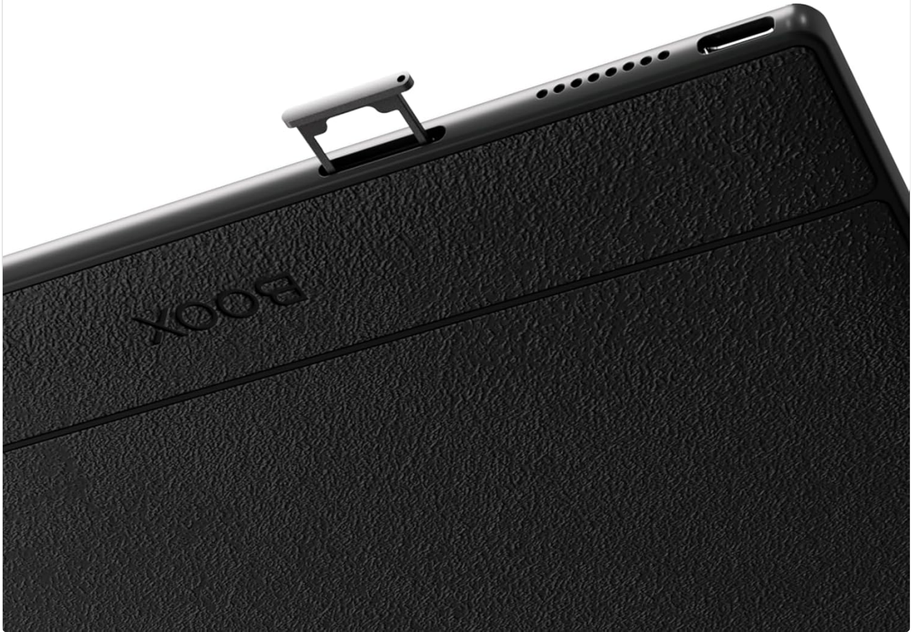
Figure 4.3: Detailed view of the top edge of the BOOX Go Color 7 Tablet, showing the microSD card slot for expandable storage and the speaker grille.
