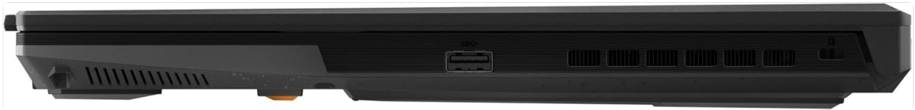
Image: The right side of the ASUS TUF Gaming A16 laptop, featuring an additional USB-A port and a headphone/microphone combo jack.
