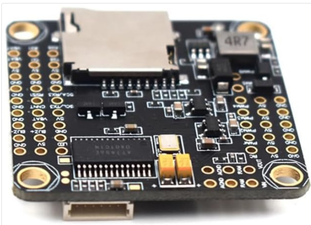
Image: Bottom view of the F4V3S Flight Controller, featuring the SD card slot for blackbox logging and additional
