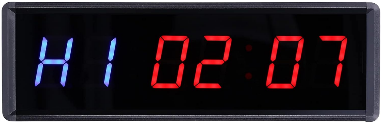
Figure 5.1.1: Timer in Clock Mode (H1 for 24-hour display)
