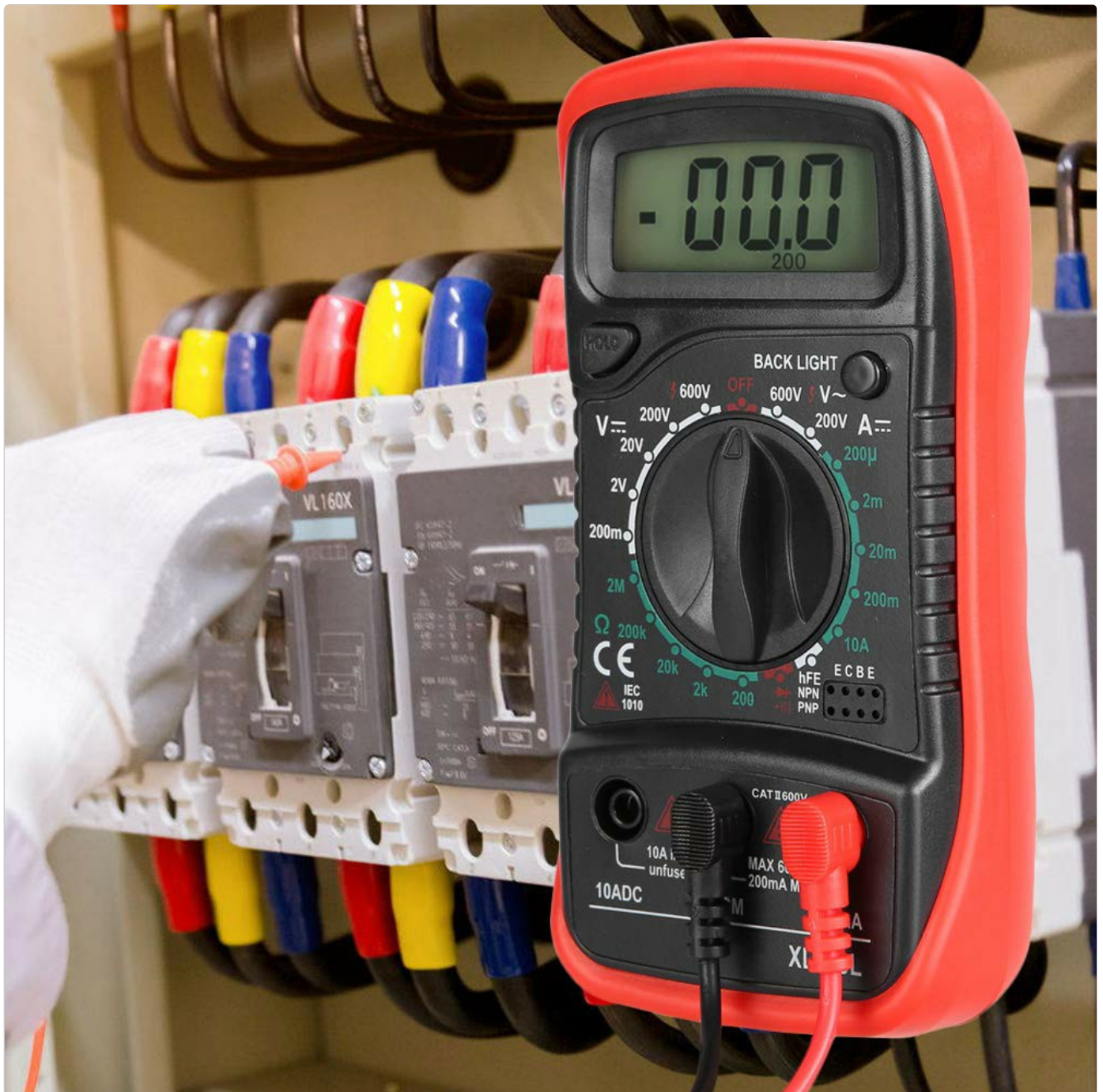
Image: A PerGar XL830L digital multimeter being used to measure components within an electrical panel. The multimeter's display shows a reading, and the test leads are connected to various terminals.
