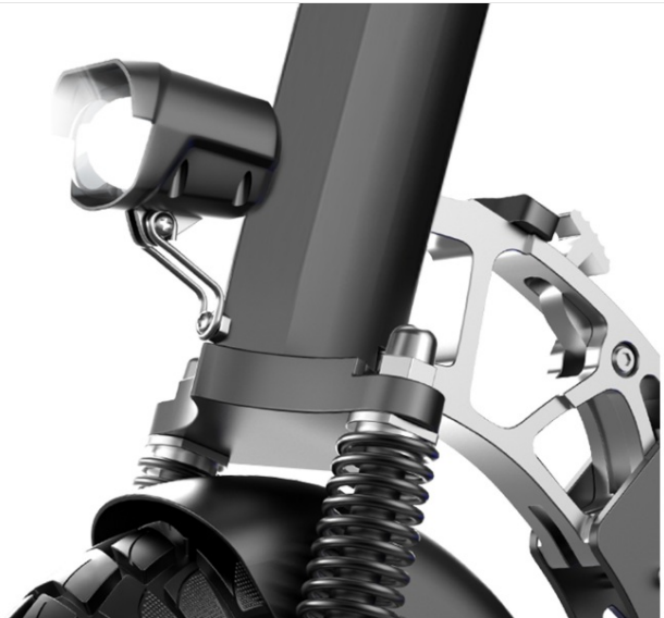
Figure 5: The dual shock absorption system provides a smoother ride.
