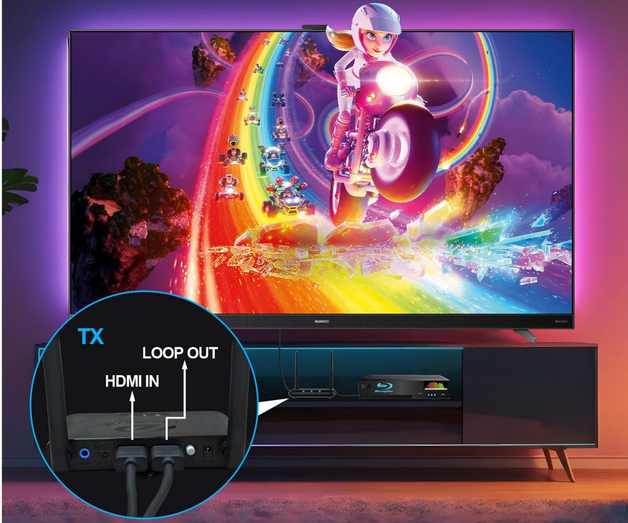
Figure 5: HDMI Loop-out function allows you to add an extra screen for the transmitter, providing local viewing while broadcasting wirelessly.
