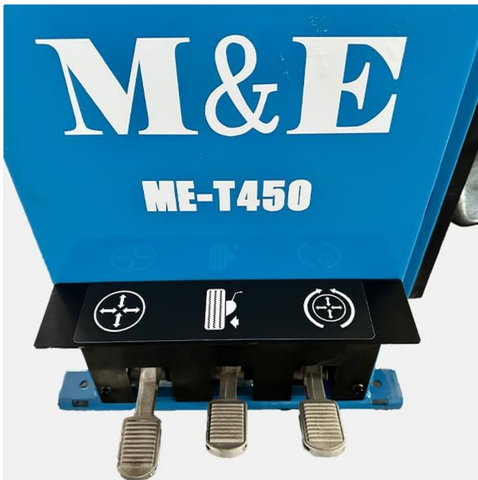
Figure 5: The foot pedals control various functions of the tire changer, including clamping, bead breaking, and turntable rotation.
