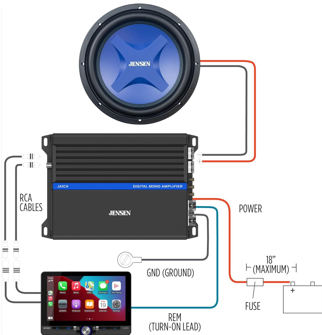
Image: A detailed wiring diagram illustrating the connection of the Jensen J4W12 subwoofer to a digital mono amplifier, which is then connected via RCA cables to a car head unit, and power/ground/remote wires to the car battery.
