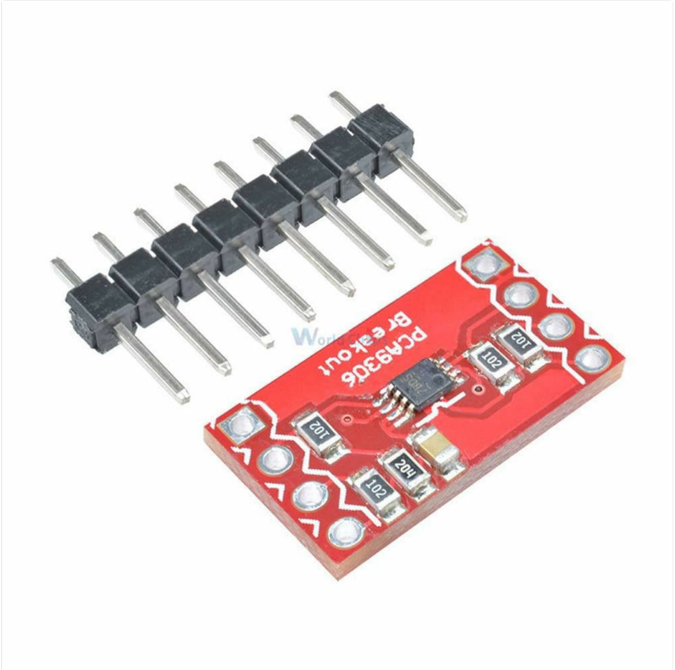
Figure 2: PCA9306 breakout board with included header pins, ready for integration into a breadboard or custom PCB.
