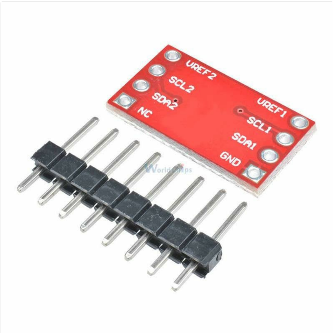
Figure 1: Back view of the PCA9306 breakout board, illustrating the pin labels for connection.
