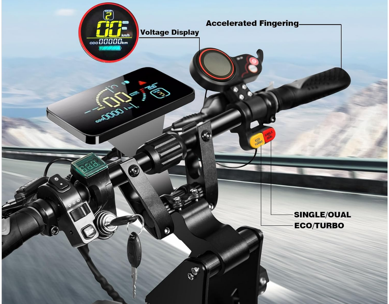
Image 4.1: A detailed view of the upgraded LCD screen and handlebar controls, including the voltage display, accelerated fingering throttle, and buttons for single/dual motor and eco/turbo modes.
