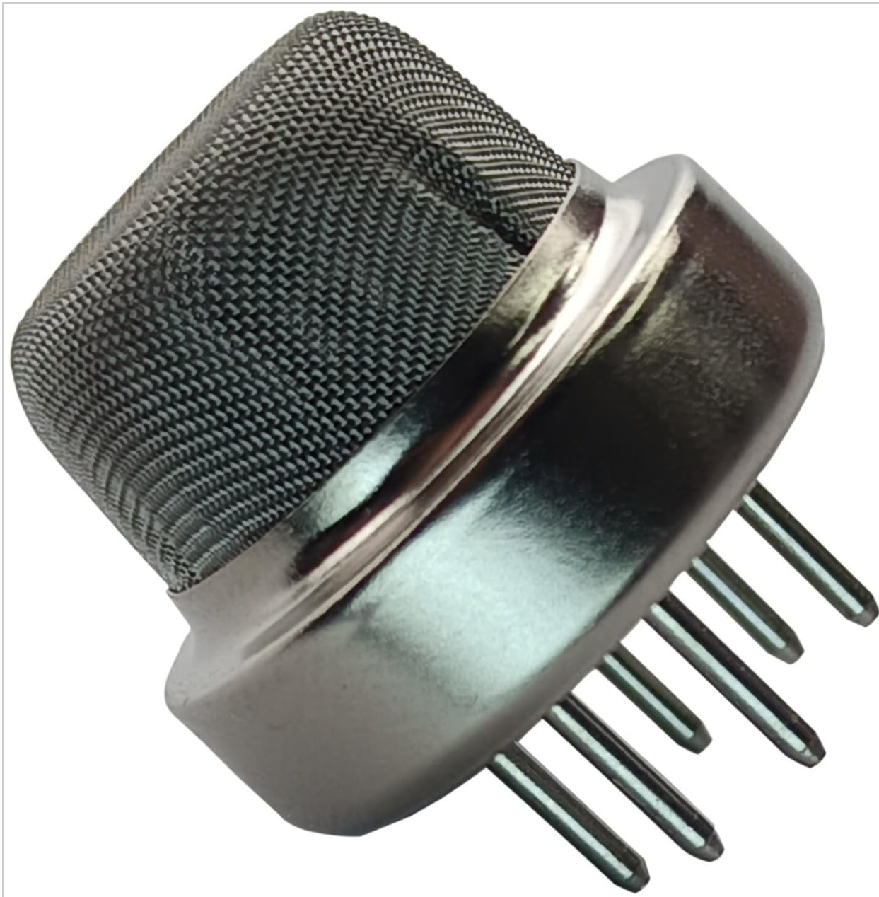
Figure 2.1: Close-up view of the WB24X799 Steam Gas Sensor, showing its metallic mesh cap and electrical pins.
