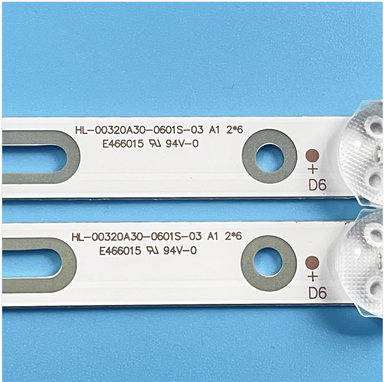
Image 3.2: Detail of a backlight strip showing the identification number HL-00320A30-0601S-03.
