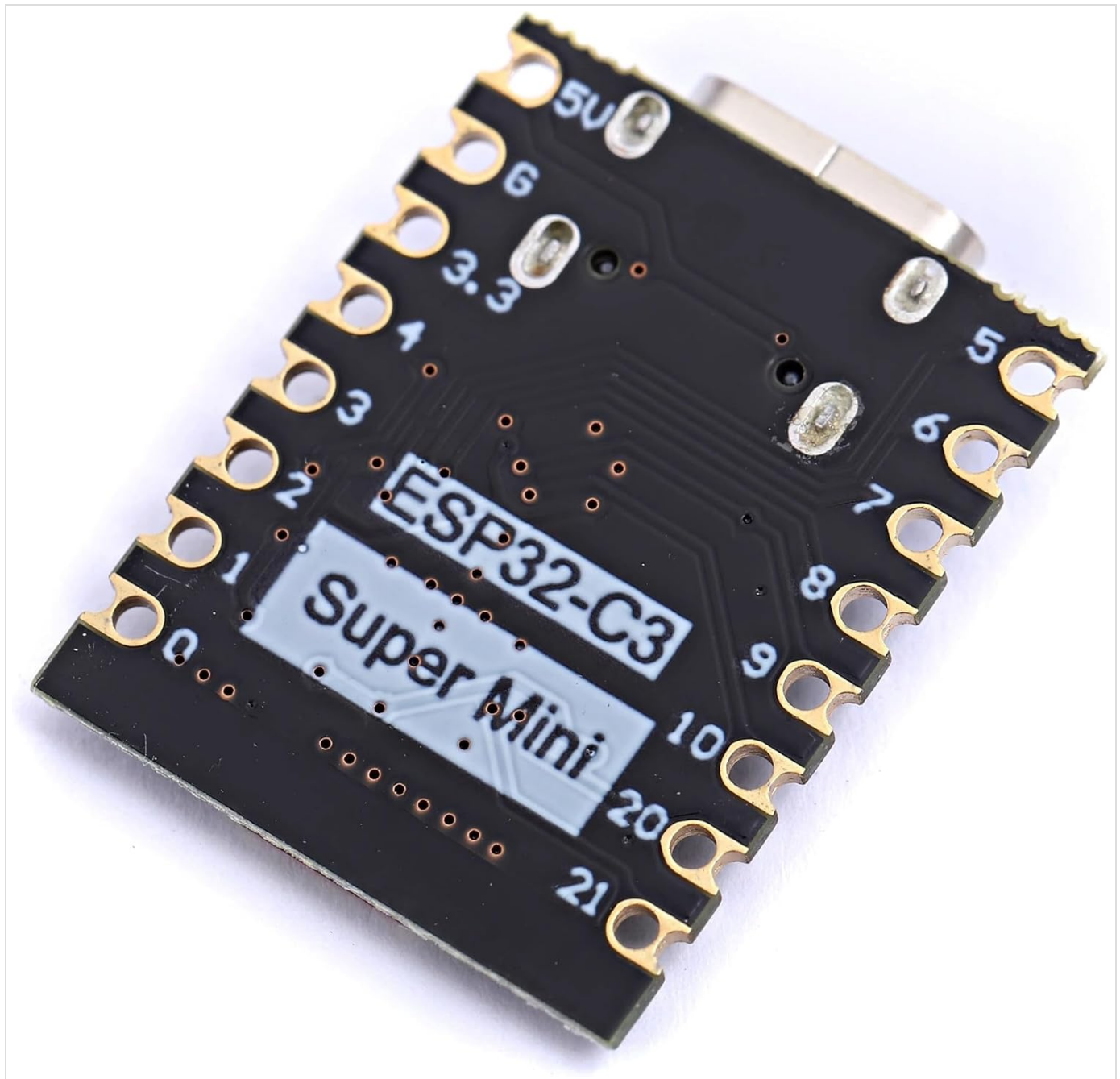
Image 3.3: Bottom view of the board, indicating pin labels and the "Super Mini" designation.
