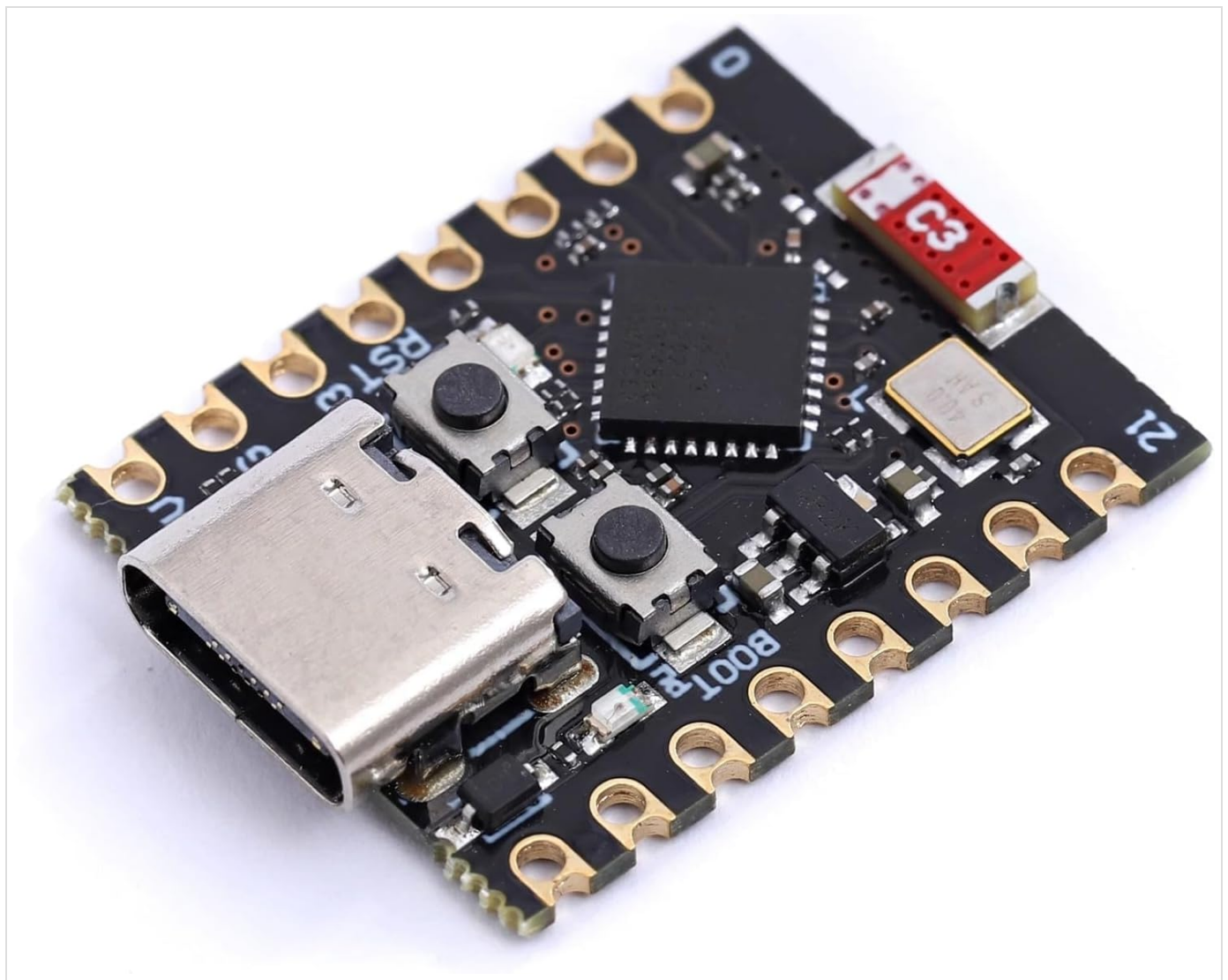
Image 3.1: Top view of the ESP32-C3 Supermini Development Board, showing the USB-C connector and control buttons.
