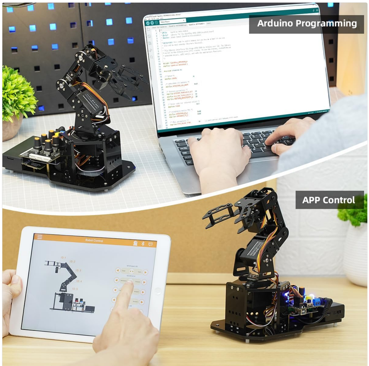
Figure 6.1: Control methods for the miniArm, including Arduino Programming and APP Control.
