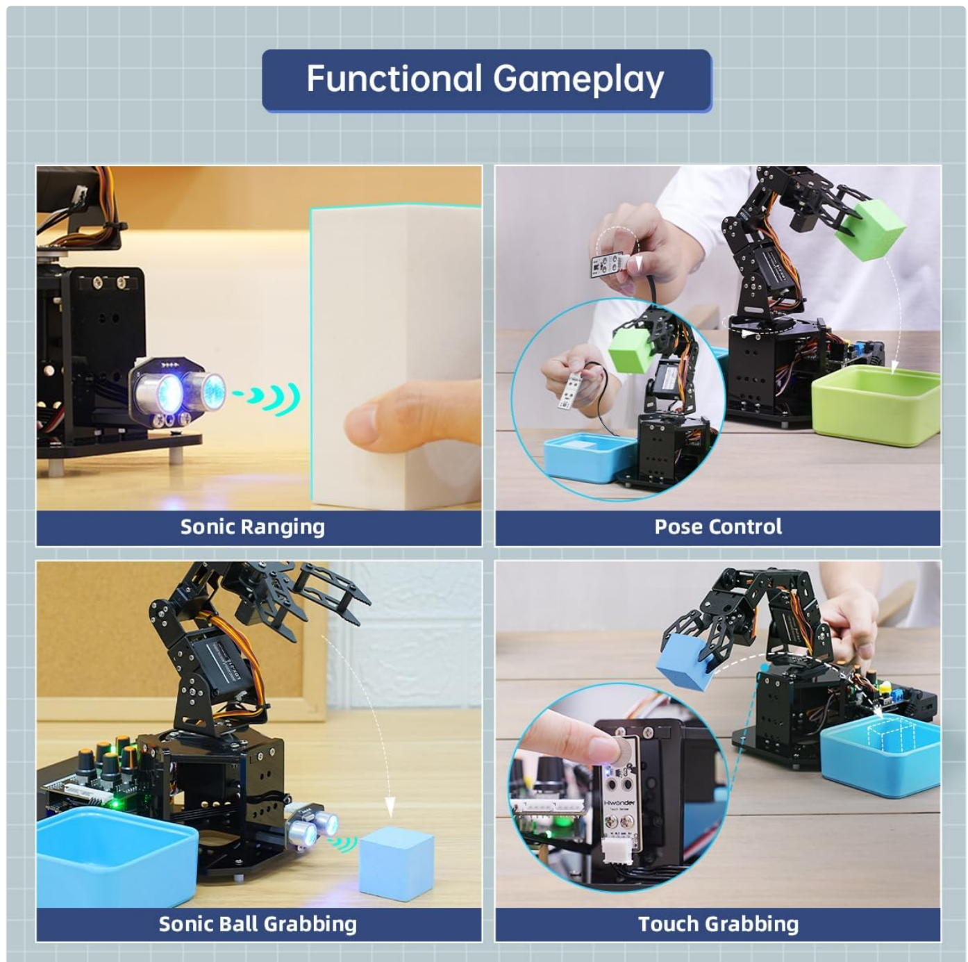
Figure 7.1: Functional Gameplay examples including Sonic Ranging, Pose Control, Sonic Ball Grabbing, and Touch Grabbing.
