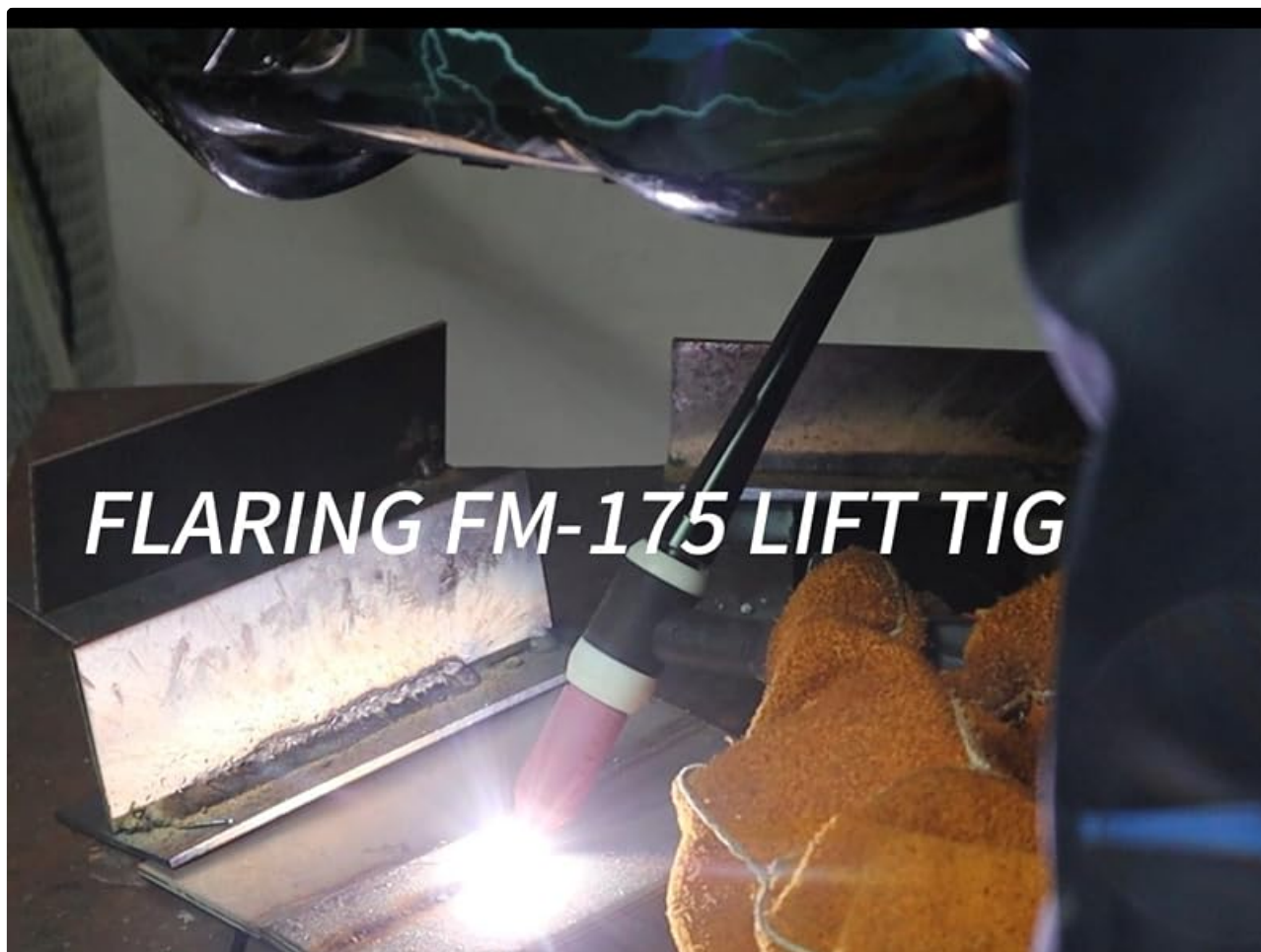
Figure 5.5: Demonstrating Lift TIG welding with the FLARING FM-175.
