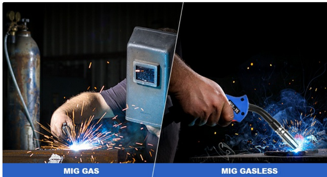
Figure 5.2: Comparison of MIG Gas and MIG Gasless welding processes.
