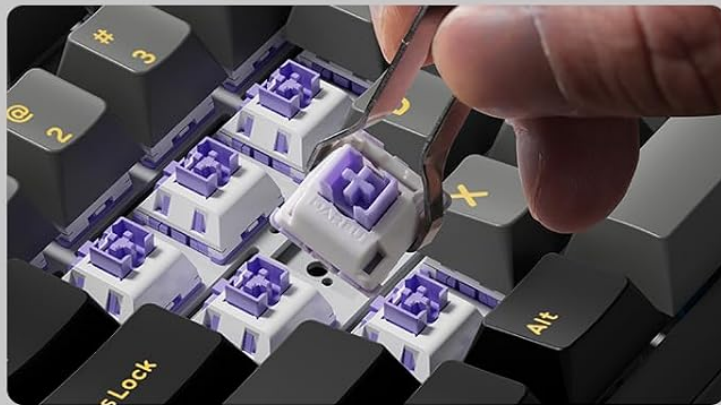
Figure 4.4: The hot-swappable PCB allows for easy switch replacement.
