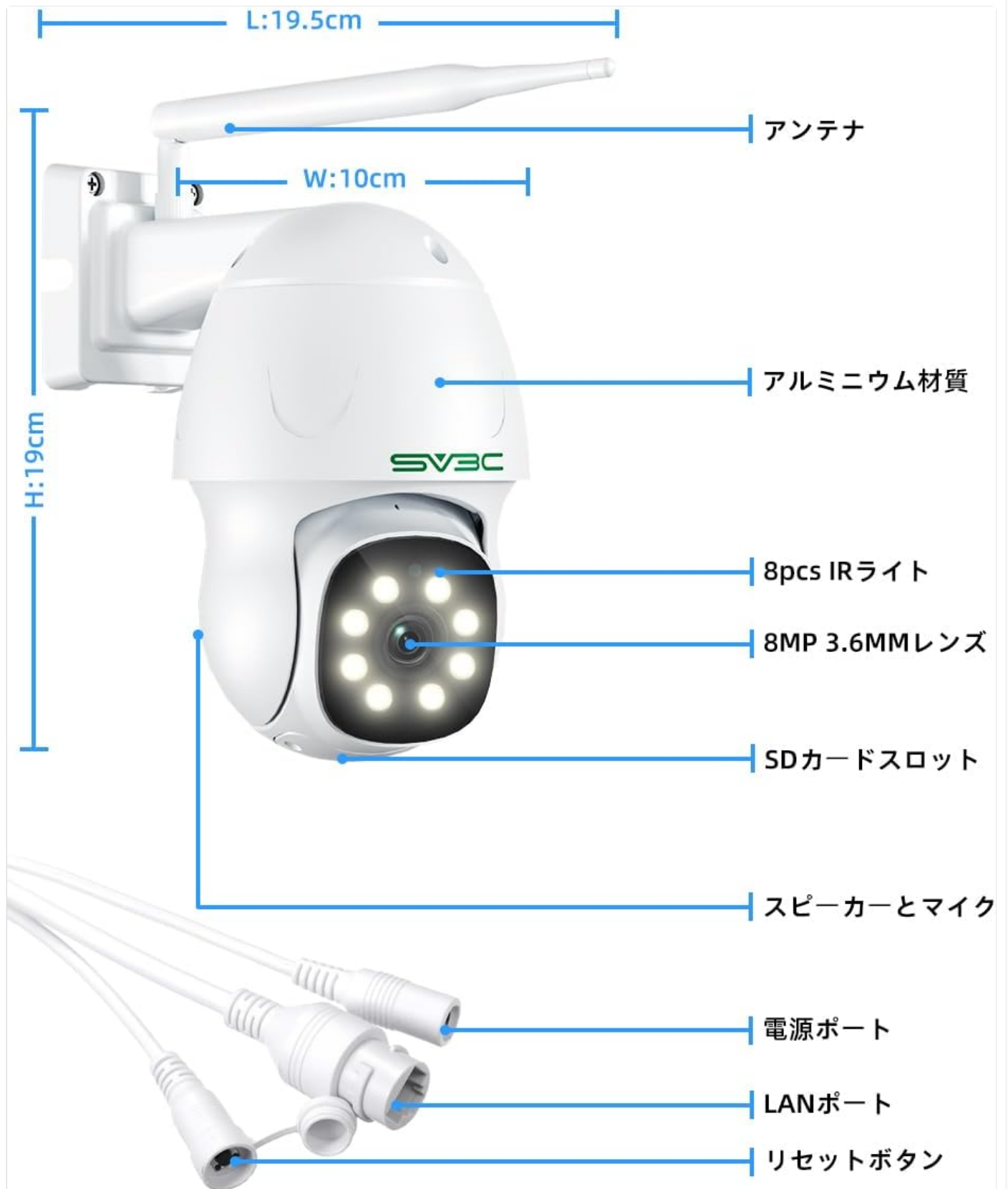
Figure 1: SV3C HX02 Camera Components. This diagram labels the antenna, aluminum casing, 8 IR lights, 8MP 3.6mm lens, SD card slot, speaker, microphone, power port, LAN port, and reset button.
