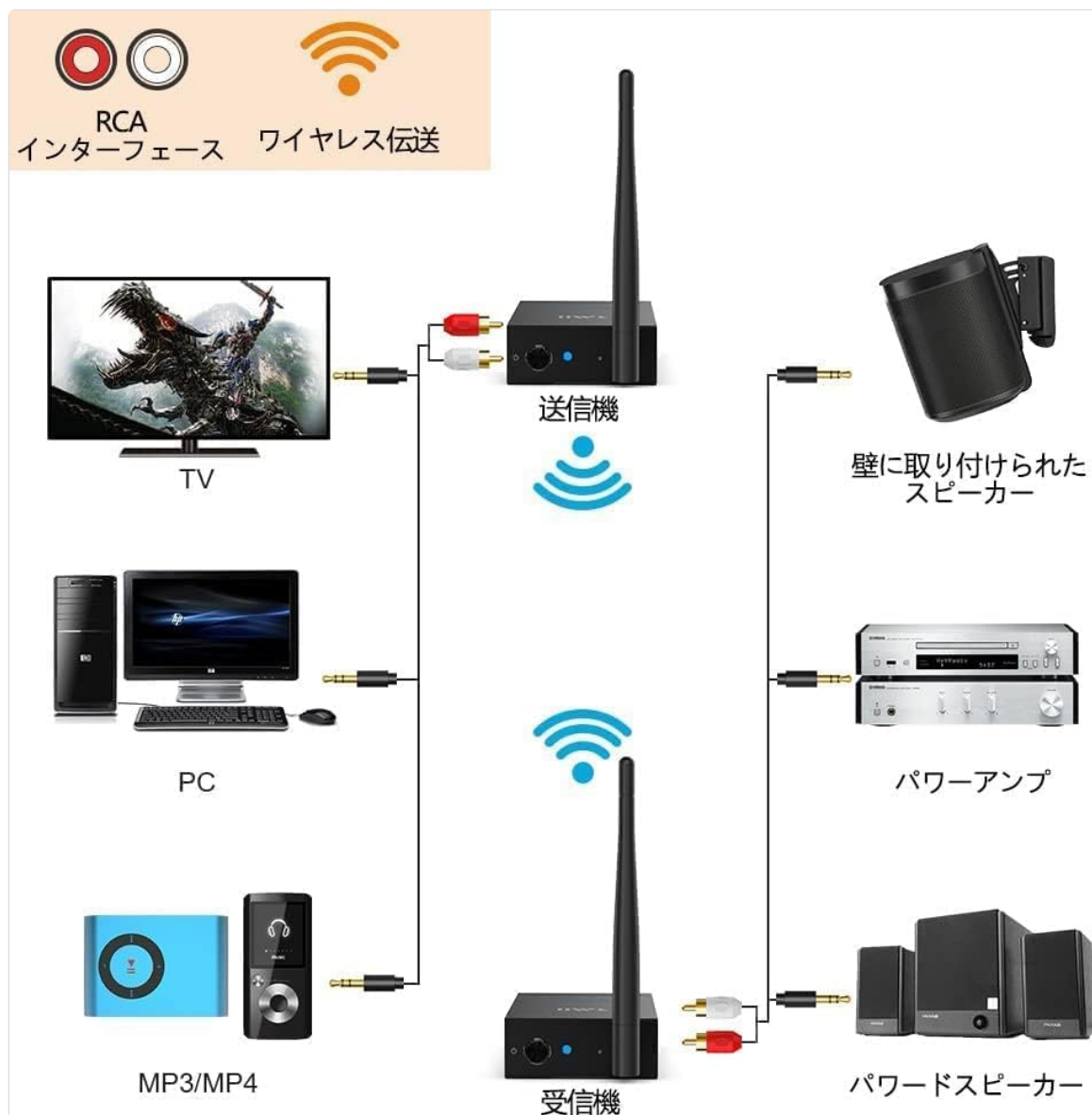
Image: Diagram showing the 1Mii Transmitter connected to a TV and PC, illustrating RCA input connections.
