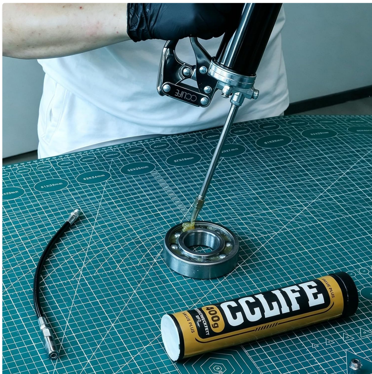
Figure 3: Applying grease to a bearing using the CCLIFE grease gun.
