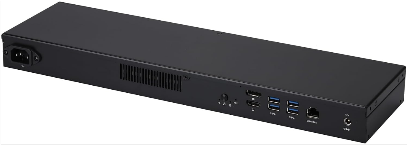
Image 3.2: Rear view of the Qotom Q1015GE-1U Rackmount Server, displaying the power input, USB ports, HDMI, DisplayPort, and console port. The rear panel includes the AC power input, four USB 3.0 ports, HDMI and DisplayPort outputs for display connectivity, and an RJ45 console port for serial management.
