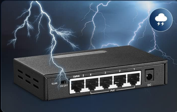
4KV Lightning Protection
