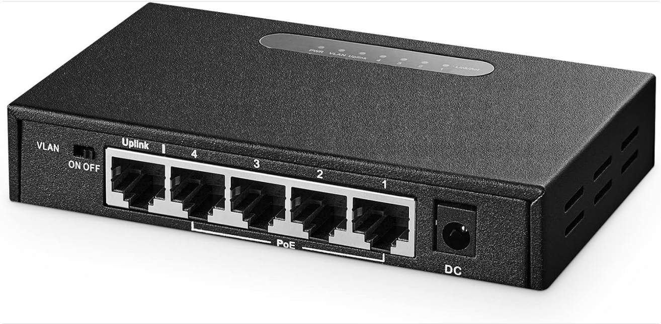
Figure 1: Top-down view of the Binardat 5-Port Gigabit PoE Switch. The device features a compact black metal casing with LED indicators on the top panel and ports on the front.
