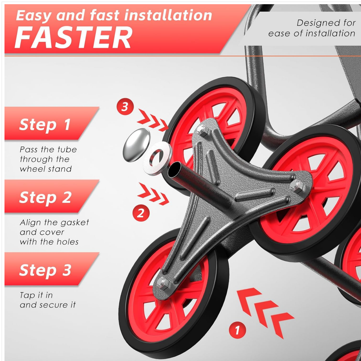
Figure 2: Visual guide for attaching the six-wheel climbing mechanism to the hand truck frame. This image illustrates the three-step process for secure assembly.
