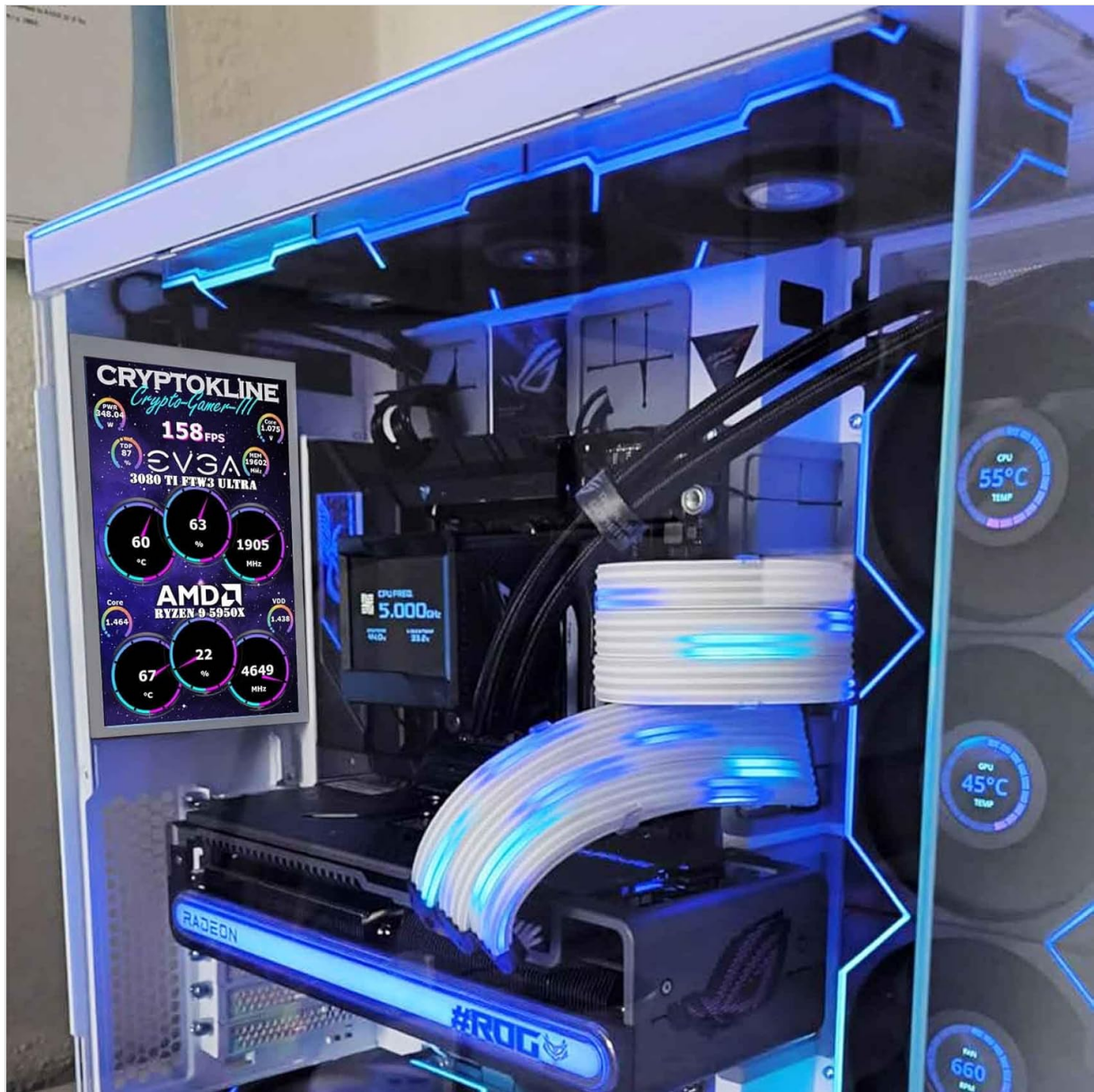
Figure 4.2: Monitor installed inside a PC case, showing system statistics.
