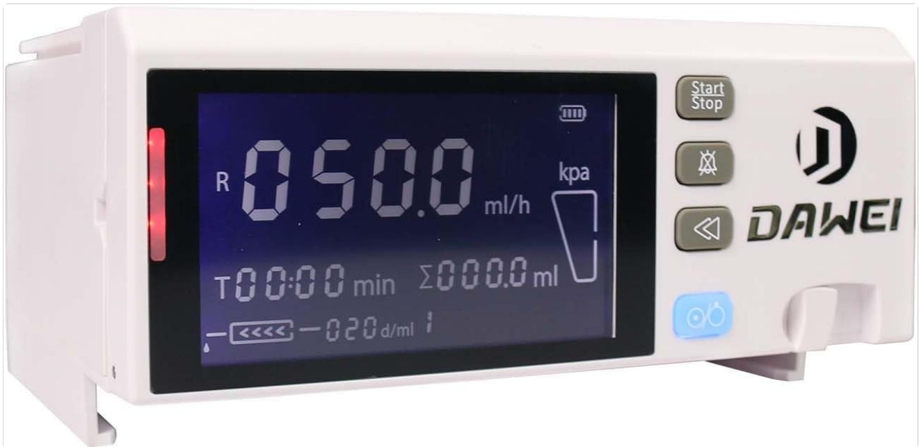
Figure 6: The AIP100 pump indicating an alarm condition with a red warning light.
