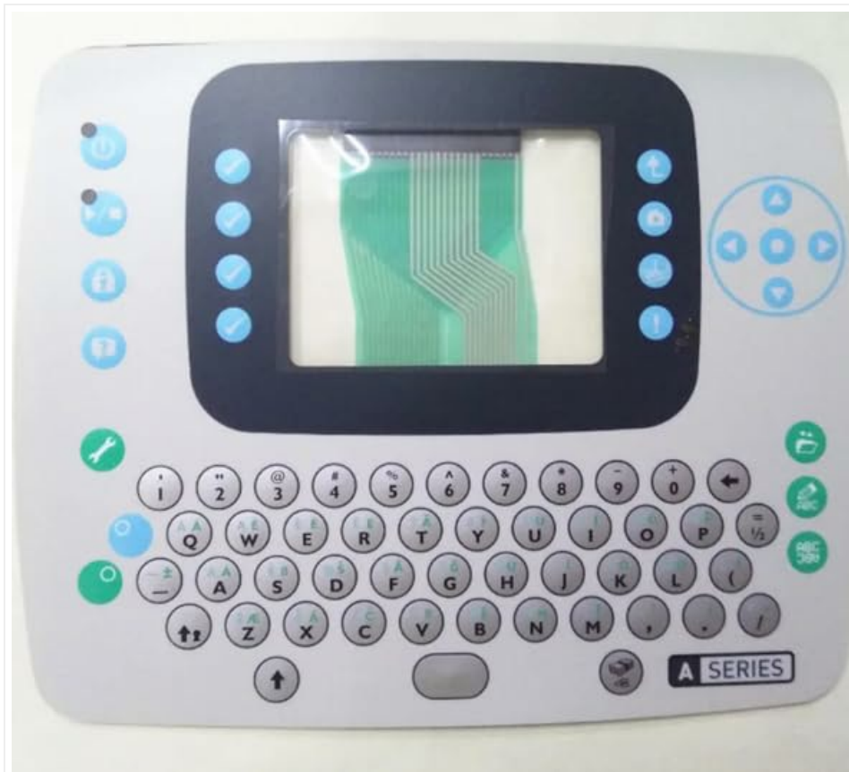
Figure 1: The Cijprinter Domino A320 A420 i-tech Keyboard Display unit. This white unit features a central rectangular
