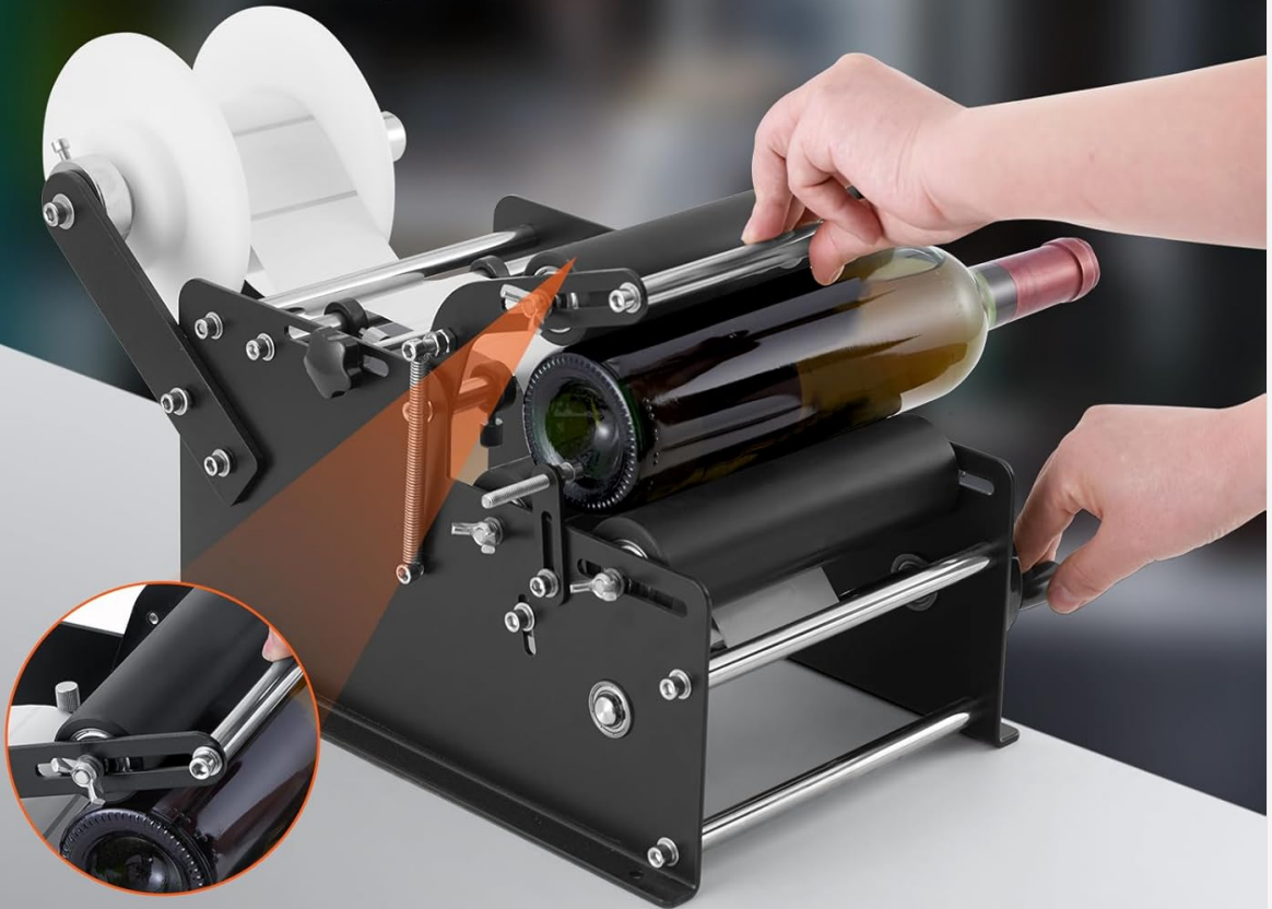
Figure 6: Applying a label using the machine's hand crank and press bar.
