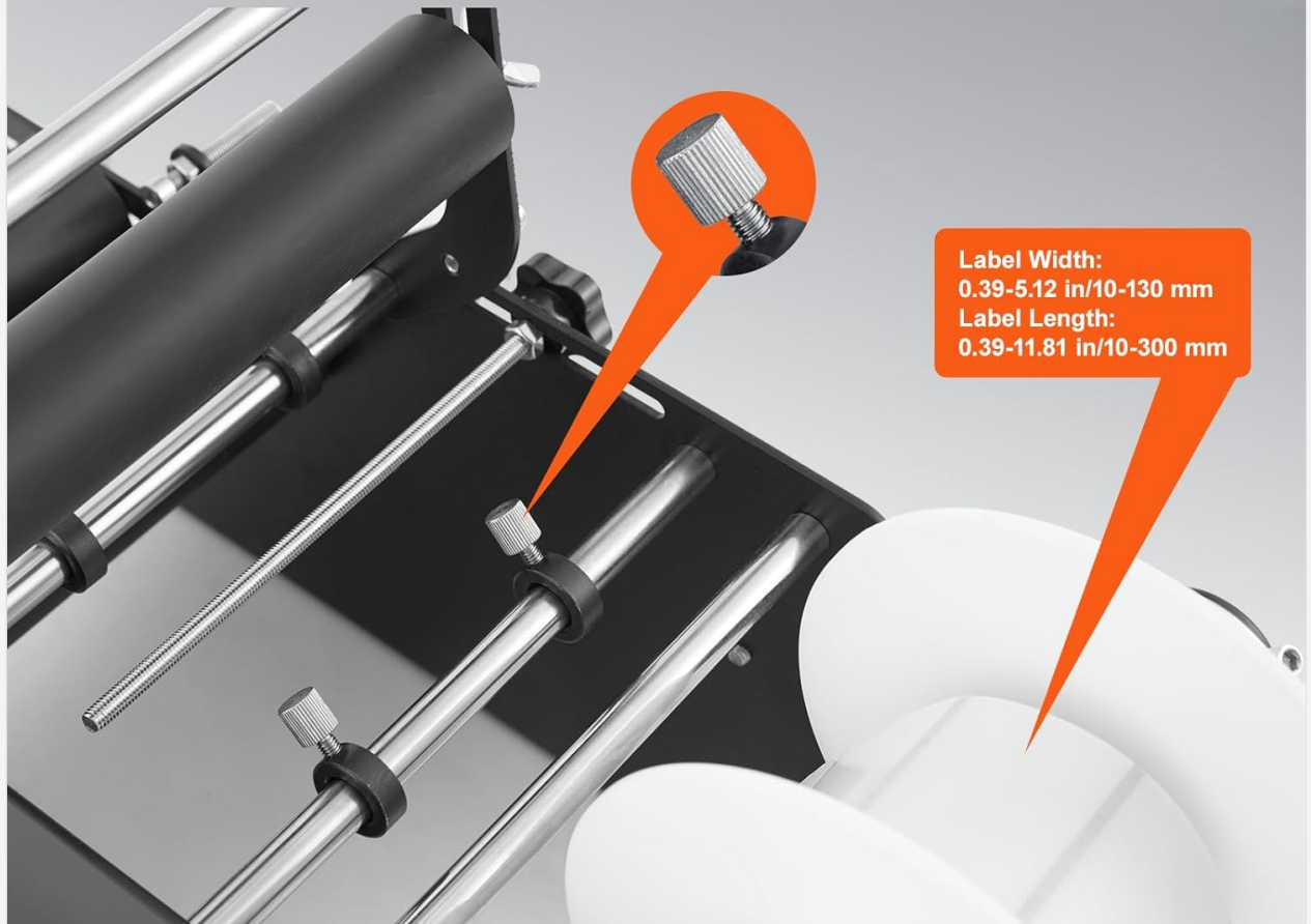
Figure 4: Detailed view of the screw adjustment for label dimensions.
