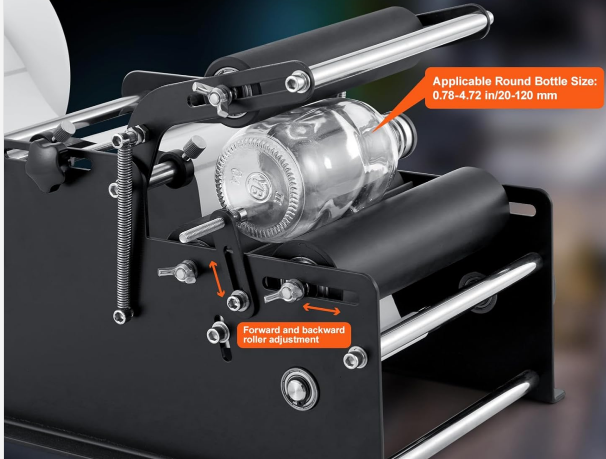
Figure 5: Adjusting rollers to fit different bottle diameters.
