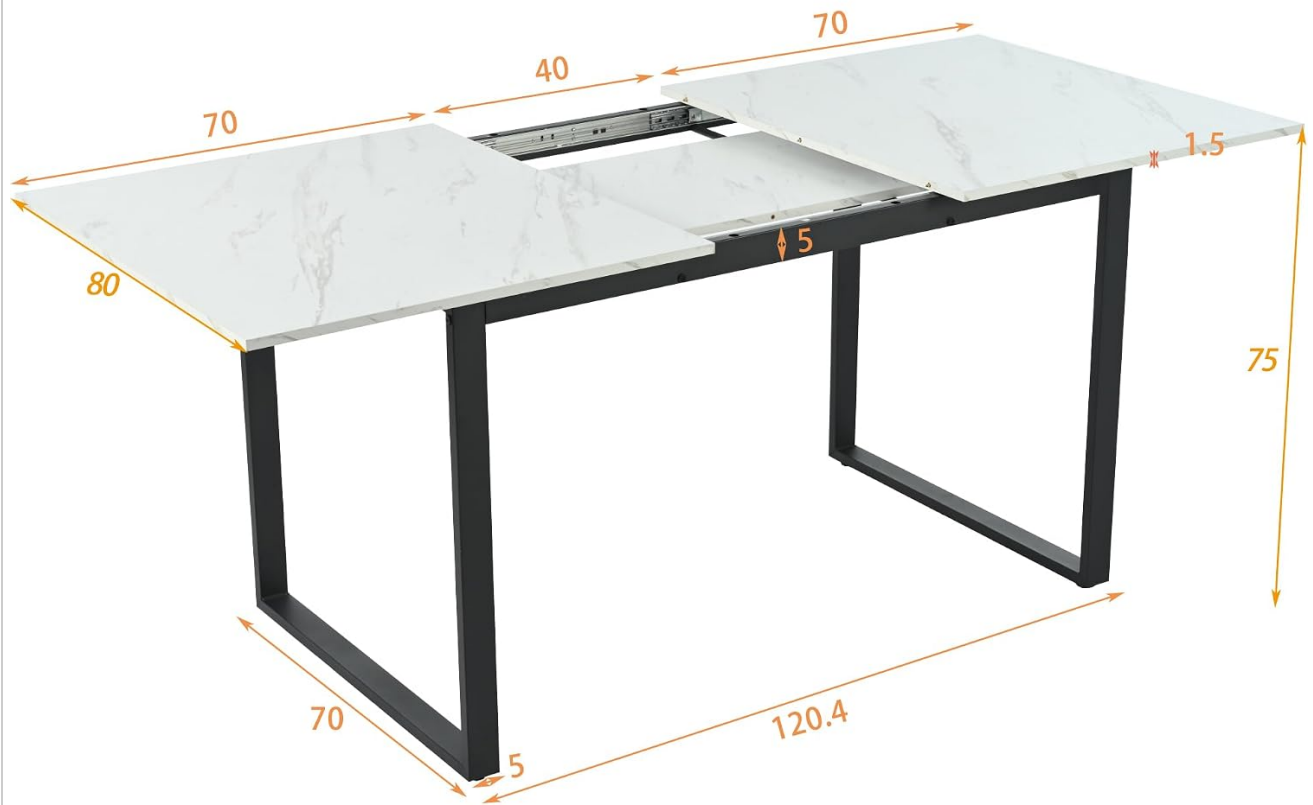
Image 4.2: Dimensional diagram of the table, illustrating its extendable nature and overall measurements.
