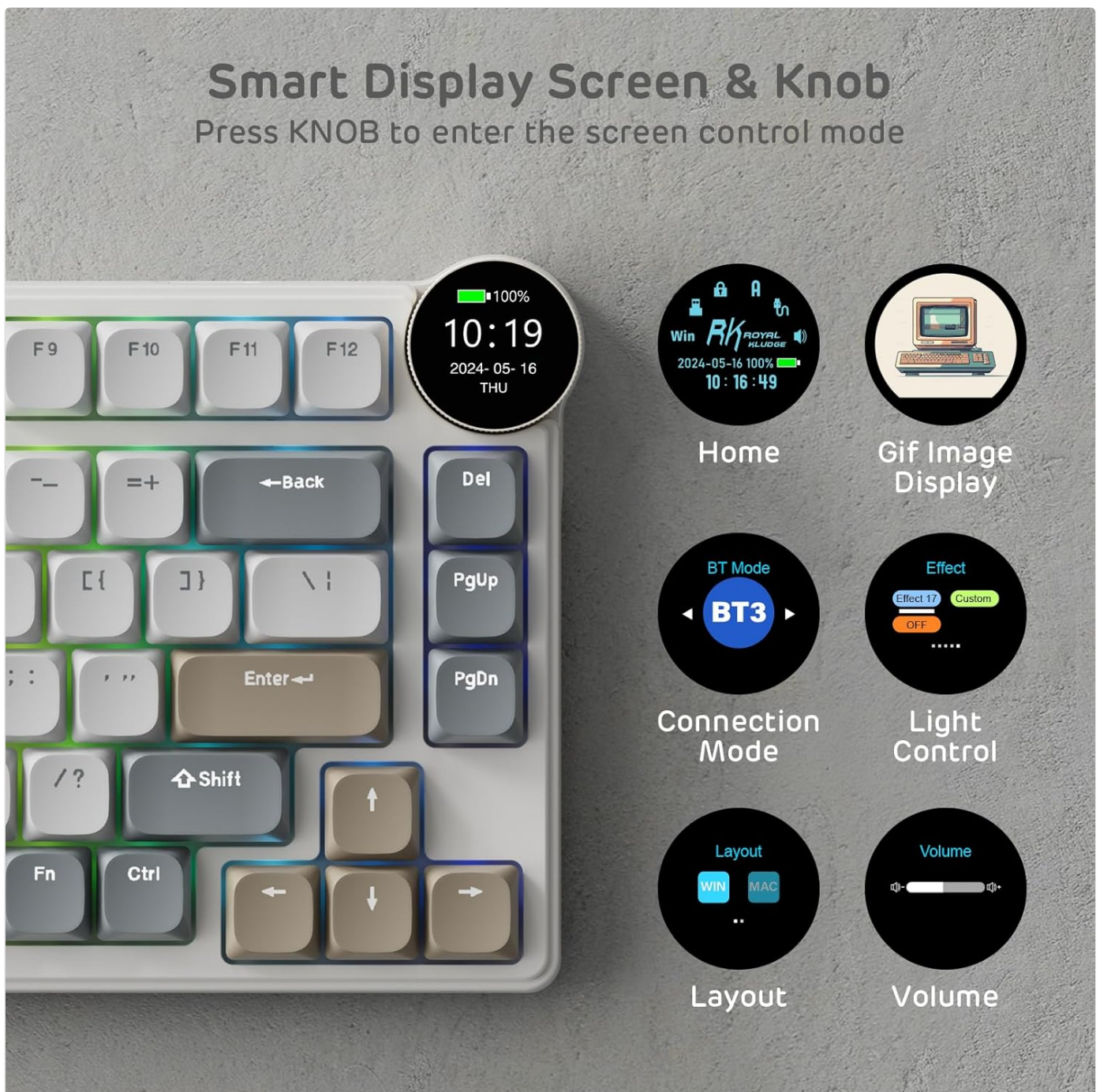
Image: A detailed view of the smart display screen and knob, illustrating the various functions accessible by pressing the knob, including home screen, GIF display, connection modes, light control, layout, and volume.
