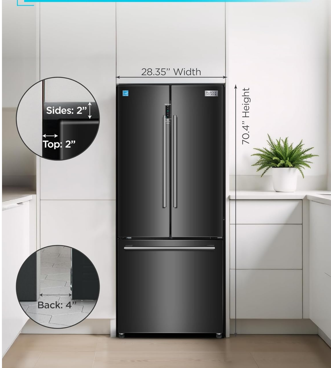
Image 3.1: Diagram showing the refrigerator dimensions (28.35" W x 29.33" D x 70.4" H) and recommended clearances: 2 inches on sides, 2 inches on top, and 4 inches at the back for proper ventilation.
