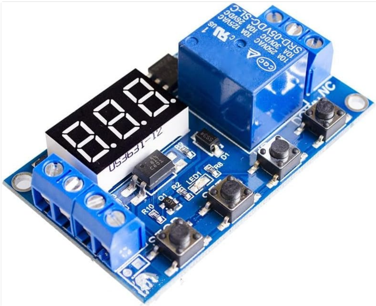
Figure 3: Top view of the XY-J02 module, showing the LED display and control buttons.
