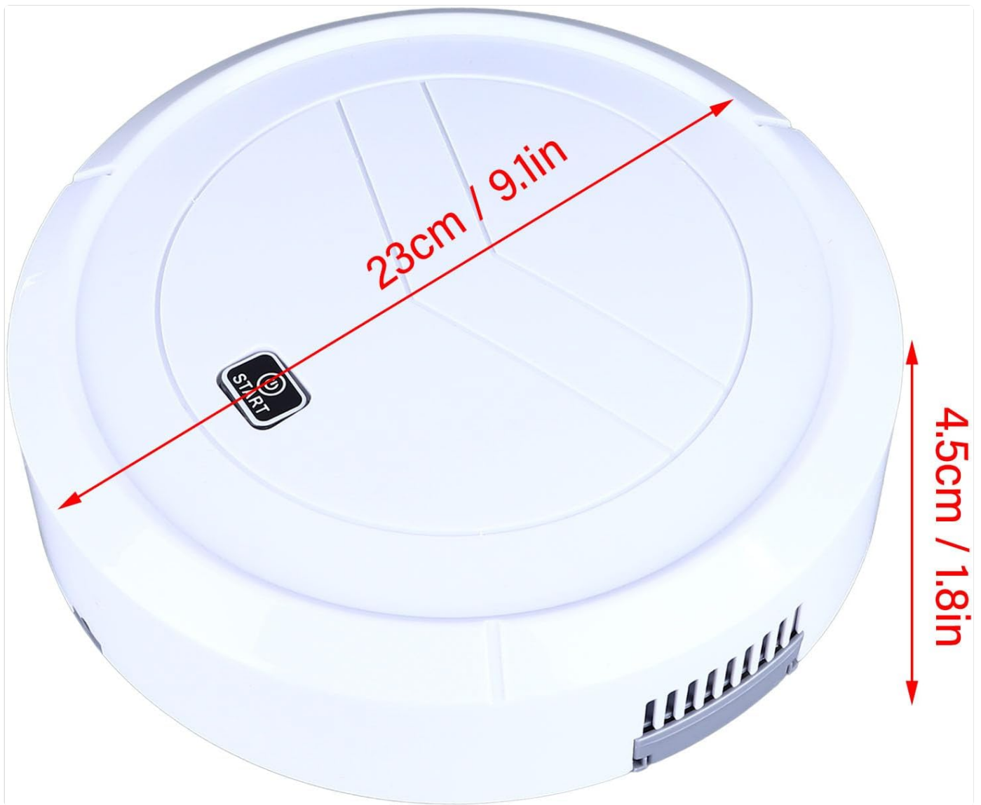
Figure 9.1: Visual representation of the robot vacuum's dimensions: 23cm (9.1 inches) in diameter and 4.5cm (1.8 inches) in height.
