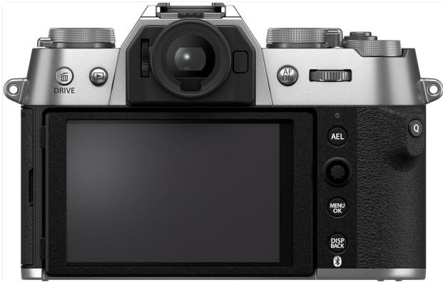
Rear view of the Fujifilm X-T50 camera body, displaying the tilting LCD screen, viewfinder, and various control buttons including AEL, Q, Menu/OK, and DISP/BACK.
