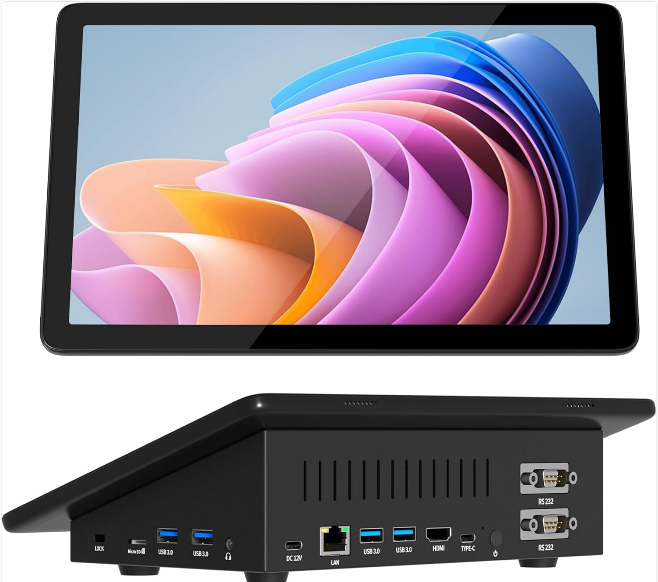
Image: Top and rear view of the HEIGAOLAPC F10 N5095 Mini PC, highlighting its integrated touchscreen and port layout.
