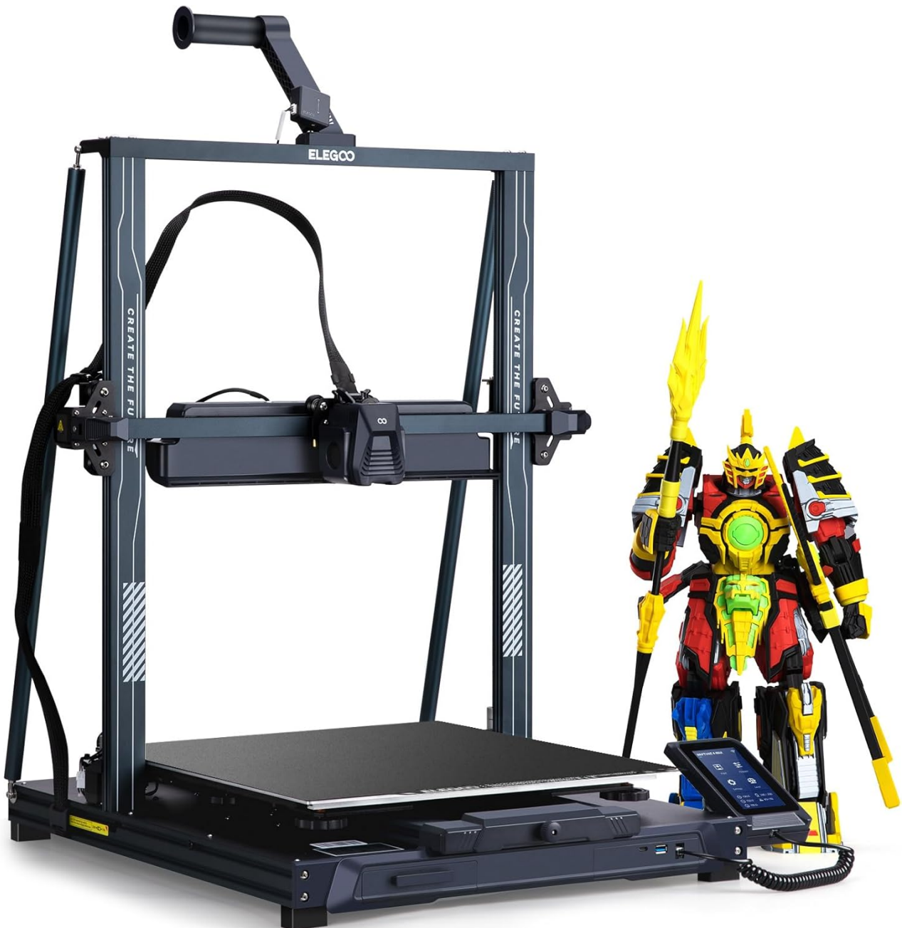
Figure 1: Assembled ELEGOO Neptune 4 Max 3D Printer. Note the large build volume and overall sturdy construction.
