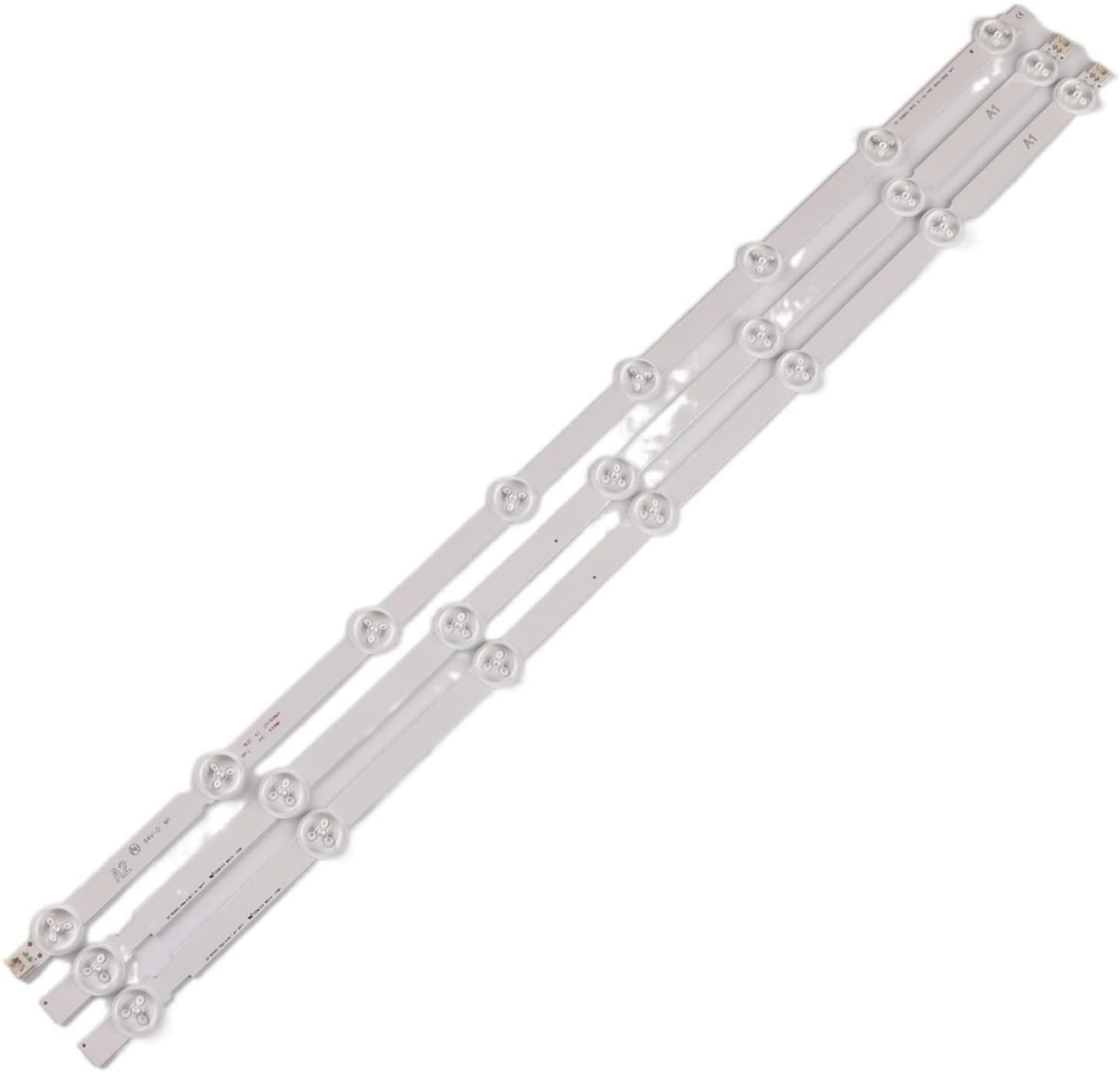
Figure 2.1: The complete set of three LED backlight strips, consisting of two A1 strips and one A2 strip, ready for installation.
