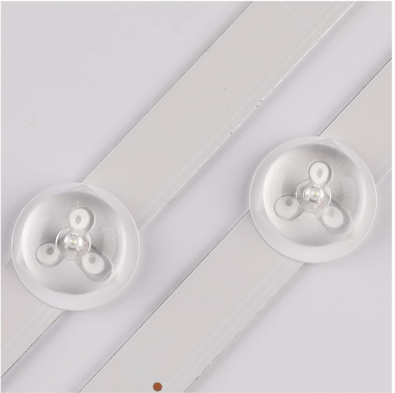
Figure 2.3: A magnified image of two LED beads, illustrating their design and placement on the backlight strip.
