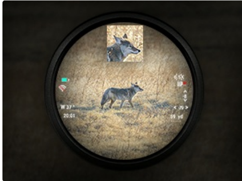
Image: The Picture-in-Picture display, showing a magnified view of the target within the main field of view.
