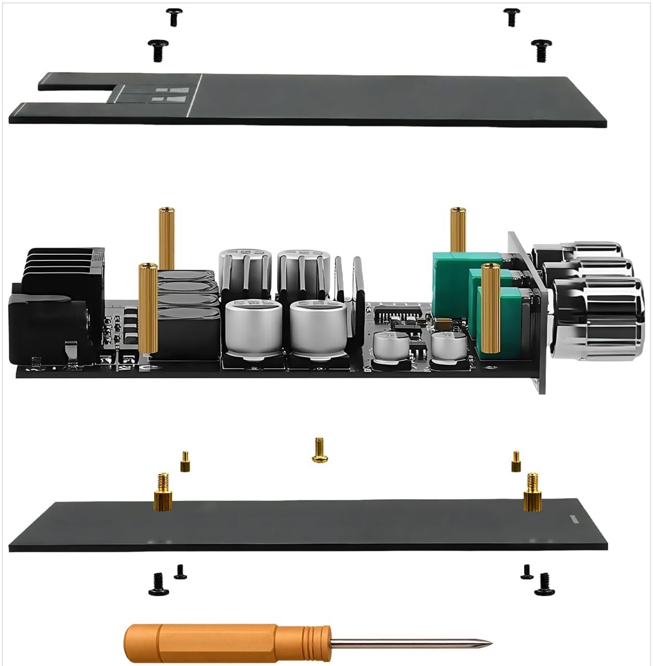
Image Description: An exploded view diagram showing the amplifier board, top and bottom case plates, brass standoffs, and screws, along with a screwdriver, illustrating the assembly process.
