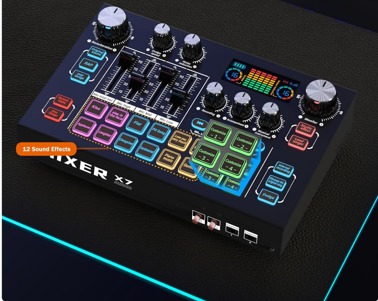
Figure 6: Overview of soundpads and internal sound effects on the RHM X7
