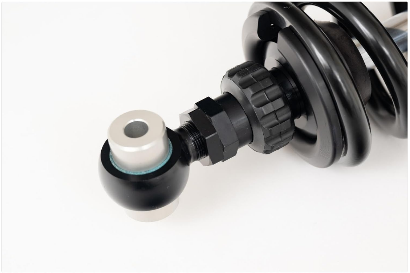
Figure 5.2: Detailed view of the OHLINS shock absorber's lower mounting point and adjustment mechanism.
