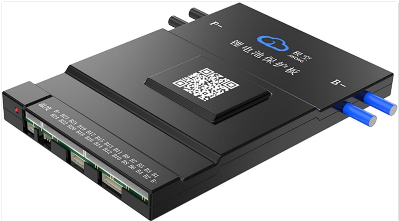
Image 5.1: Top view of the JK Smart BMS, illustrating the main power connections and balance port.
