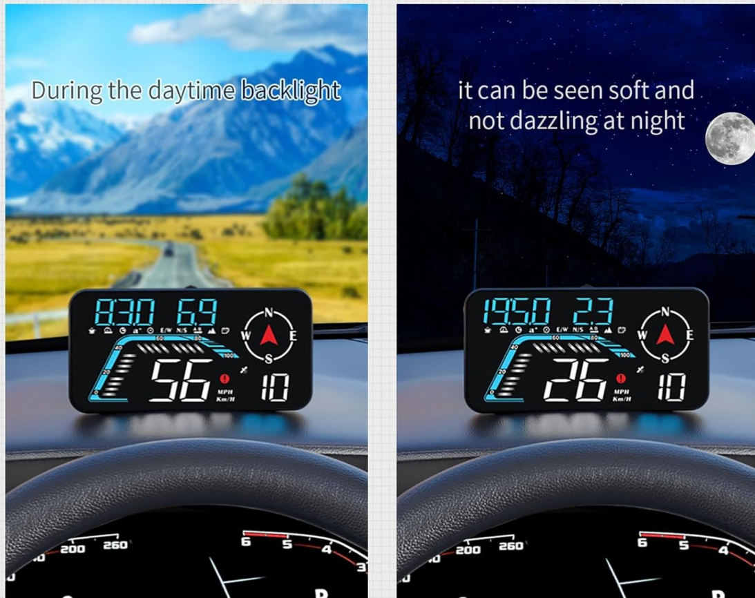
Image 6.1: Comparison of the G12 display's adaptive light sensing feature, showing clear visibility in bright daytime conditions and soft, non-dazzling illumination at night.
