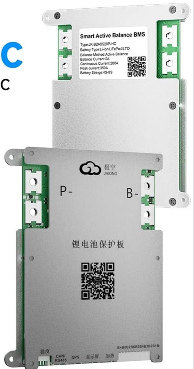
Figure 8.2: Detailed view of the Aoleaby JK Smart Active Balance BMS, model B2A8S20P-HC, showing key specifications such as 2A balance current, 4S-8S battery strings, 200A charge/discharge current, and compatibility with LiFePO 4 , Li-ion, and LTO battery types. Dimensions are also indicated.
